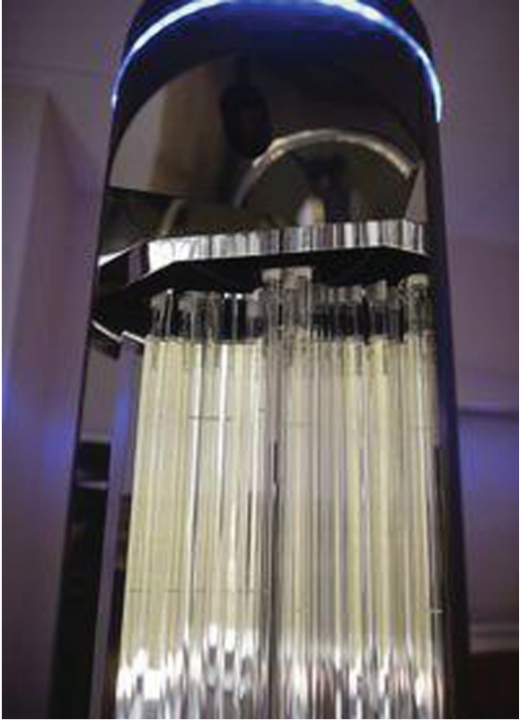
A closer look at one of the Surfacide devices when it is not in operation. When the machine is turned on, the light emitters can disinfect a patient room at Waterbury Hospital in about 30 minutes, which traditional cleaning can miss. Erin Covey / Republican-American
