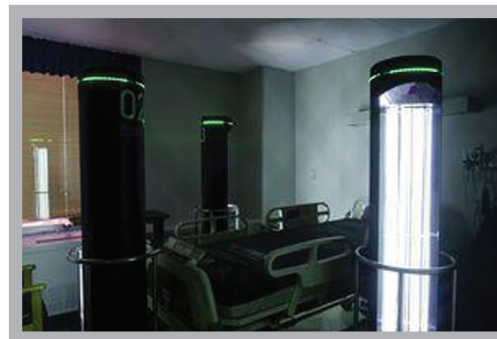
Three Surfacide light emitters slowly spin and disinfect a patient room at Waterbury Hospital during a demonstration. The three machines are able to more quickly clean common bacteria in hospitals, like C.Diff and MRSA, disinfecting a typical room in about 30 minutes. Erin Covey / Republican-American
