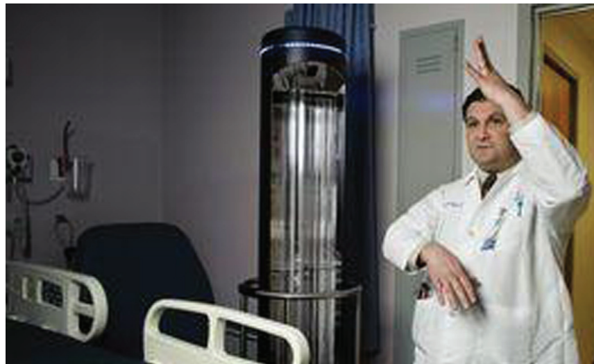
Dr. Steven Aronin, Chief of Infectious Diseases at Waterbury Hospital, explains how the Surfacide light emitters work. The devices can disinfect a typical patient room in about 30 minutes. Using three machines at one time, they are able to more quickly clean common bacteria, like C.Diff and MRSA, than traditional scrubbing. Erin Covey / Republican-American
